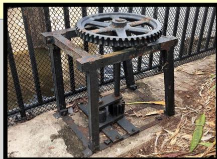
The original hand-driven rack-and-pinion mechanism used to open and close the gates
